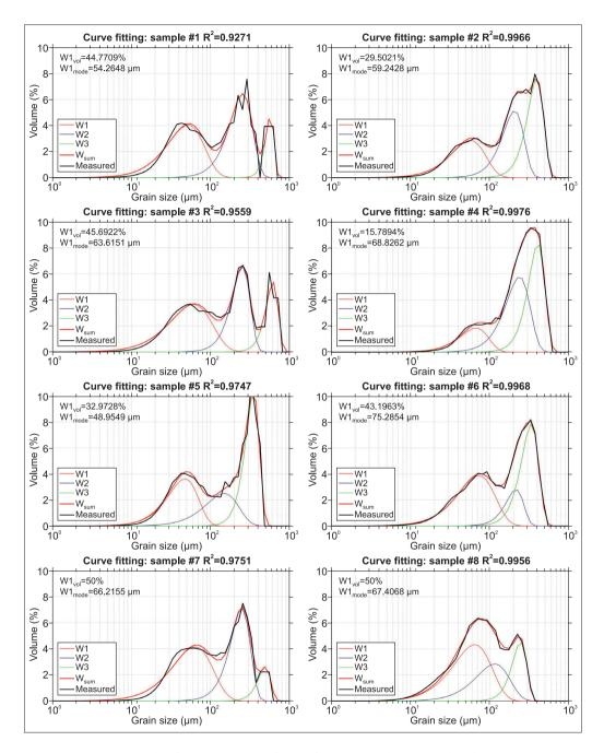
Fig. 4. Results of parametric curve-fitting of the measured grain size distributions
