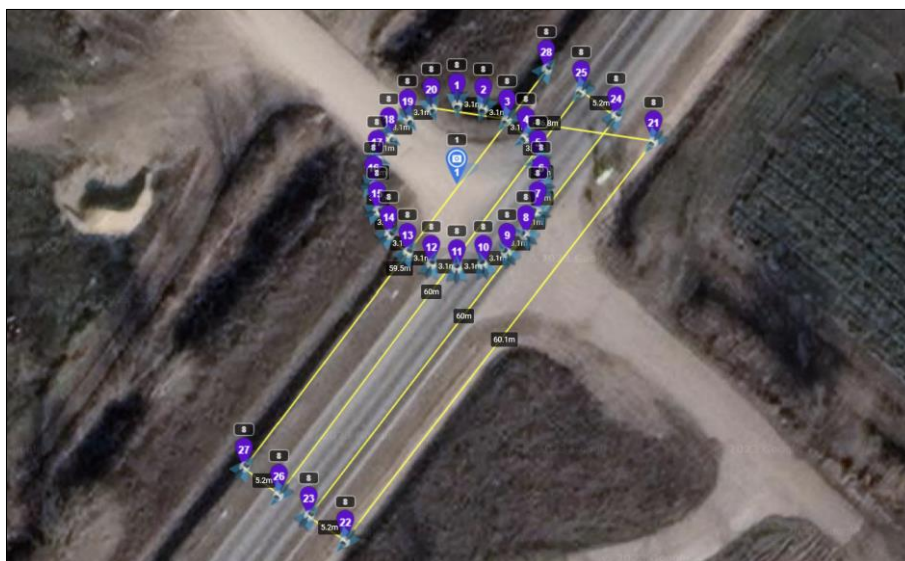
Figure 3. The route of the UAV in the test runs. Yellow lines show the route, and purple circles depict the points where the UAV changed direction. In the circular route, photos were taken at the places marked by purple circles
