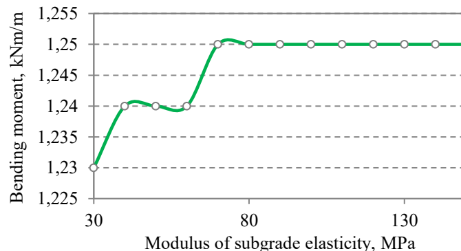
Figure 13. Dependence of bending moments in metal structures on the modulus of elasticity of the foundation soil
