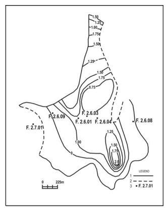
Figure 3. The IV<sup>th</sup> lignite seam isopachs at Târșolț (data by Kovács-PALFFY et al. 1982)
