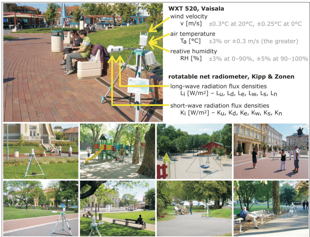
Fig. 3. Human bio-meteorological measurements and questionnaire surveys on popular recreational areas of Szeged. (Accuracy of measured parameters are also indicated).
