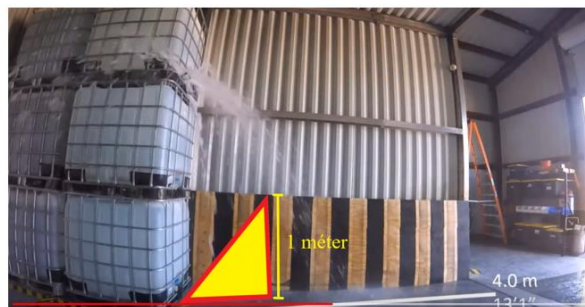
9. picture: Damage to IBC due to forklift fork, own editing by [24]
