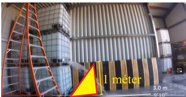
10. picture: IBC damage at the tap and due to forklift fork, own editing by [24]
