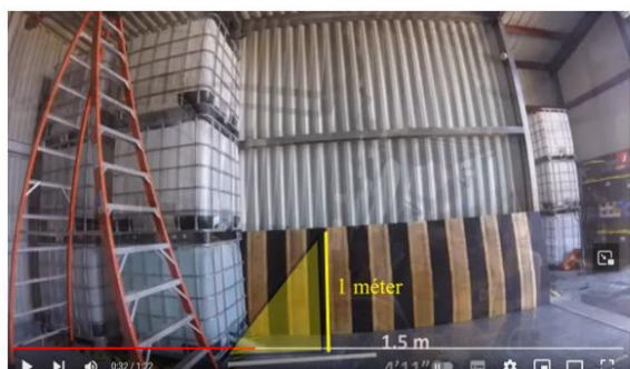
11. picture: IBC damage for one storage level, own editing by [24]
