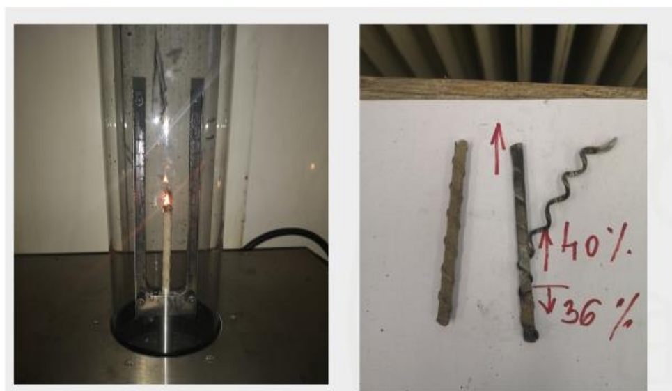
Figure 7 - Typical apparatus for the determination of oxygen index and damage to the specimens after burning in 35 and 40% oxygen. Created by the Authors.
