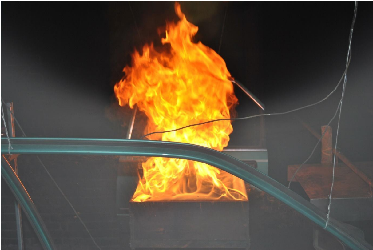
Figure 6. Flame-burning of the source on the door, window level
