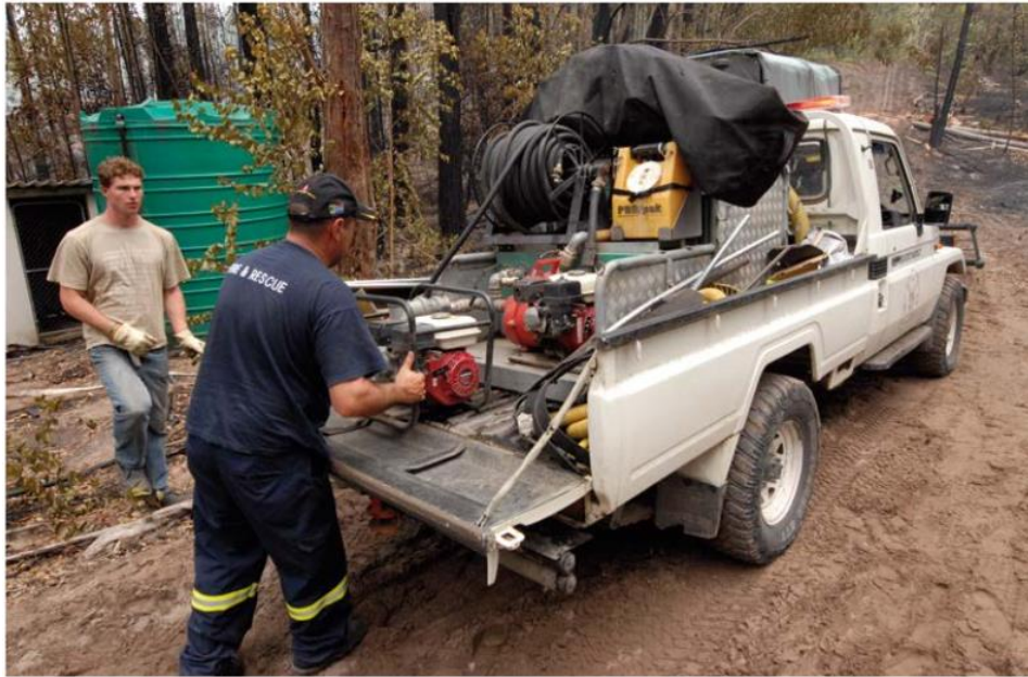
Figure 10 - A landowner vehicle fitted with firefighting equipment. Source [4].
