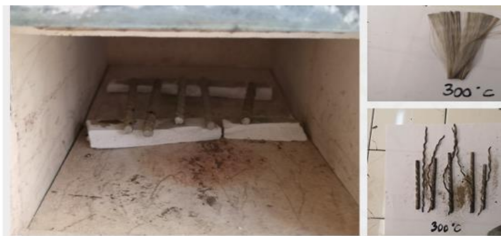
Figure 6 - Samples in the furnace before heating and the consistency of the samples after 24 hours at 300 °C. Source: Authors.
