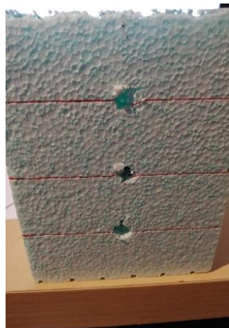
Figure 3 - Thermo elements in the specimen. Source: Authors.
